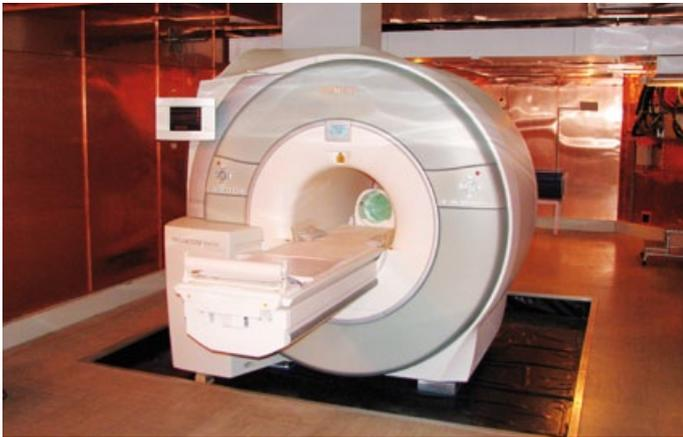
The 3-tesla whole-body tomograph at PTB's Observatory.
