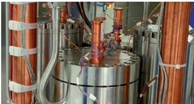
Core piece of PTB's gas thermometer for the redefinition of the kelvin: Four pressure cylinders of stainless steel accommodate the different capacitors for the measurement of the dielectric gas constant.
