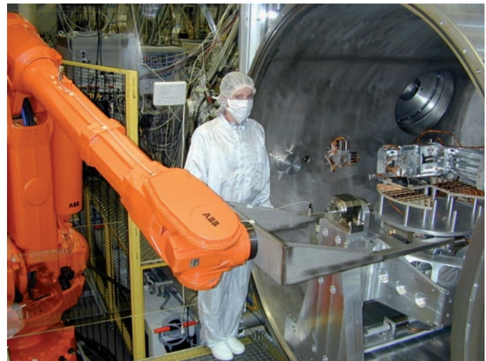
The EUV reflectometer allows optical components with a mass of up to 50 kg and diameters of up to 65 cm to be characterized.
