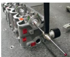
Coordinate measuring machines (CMMs) are important auxiliaries in industrial metrology. The figure shows a CMM during the calibration of a motor block which is used as a workpiece-like calibration standard in accredited calibration laboratories (DAkkS).
