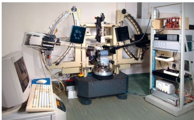
Orientation apparatus for single-crystal materials. The device is approx. two meters in height and has a weight of about two tonnes.
