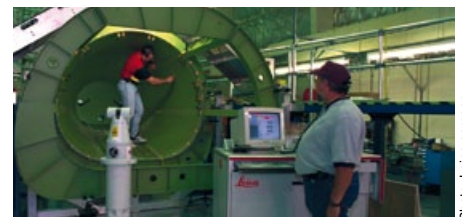
Flexible determination of large measurement ranges: Theodolite system – in the fore-ground, on the left – during use in dimensional measurements on an aircraft component.
