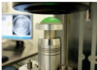
Optical form measurement with the aid of the tilted-wave interferometer.
