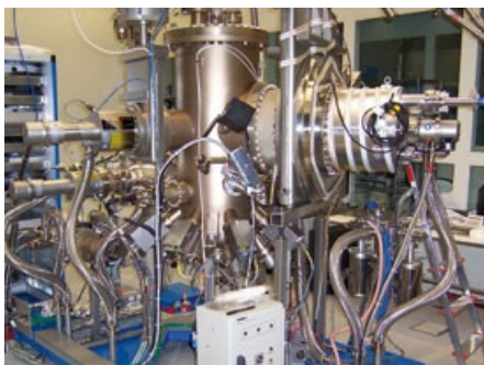
Molecular beam epitaxy machine used to manufacture semiconductor quantum standards such as quantum Hall resistors.
