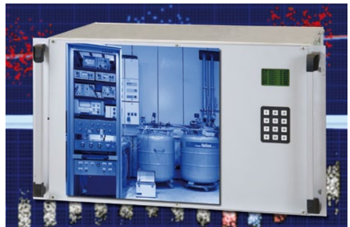
Cryogenic current comparator set-up used to compare different DC resistors in order to establish the ohm scale.
