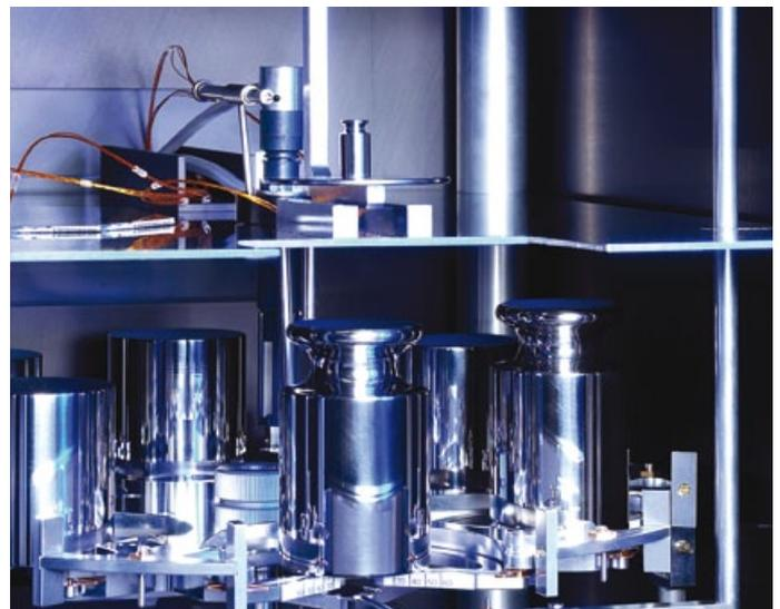
View into the proto-type balance with the aid of which 1 kg mass standards can be linked up with the national kilogram prototype.
