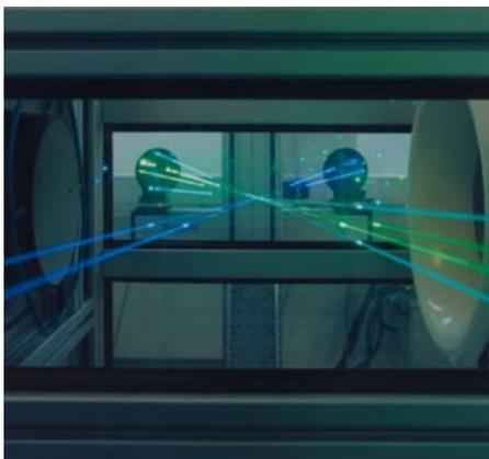
Calibration of a wind measuring device (anemometer) with the aid of Laser Doppler Anemometry.
