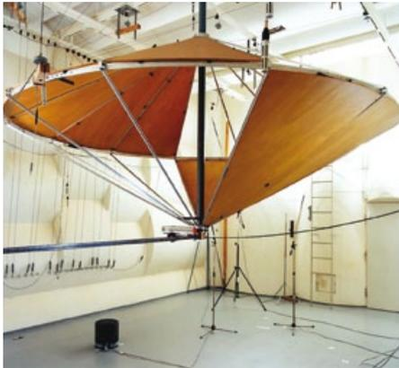
PTB's reverberation room: The rotating screen makes sure that the sound of a noise source is distributed in the room as uniformly as possible.
