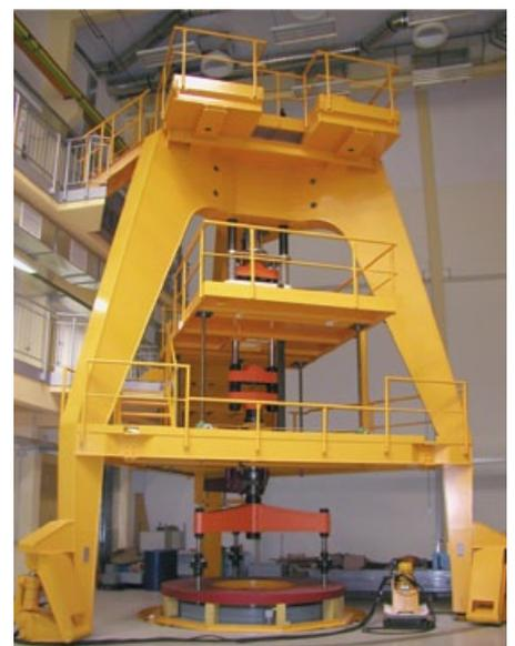
The 2 MN force standard machine is the largest deadweight machine of PTB.
