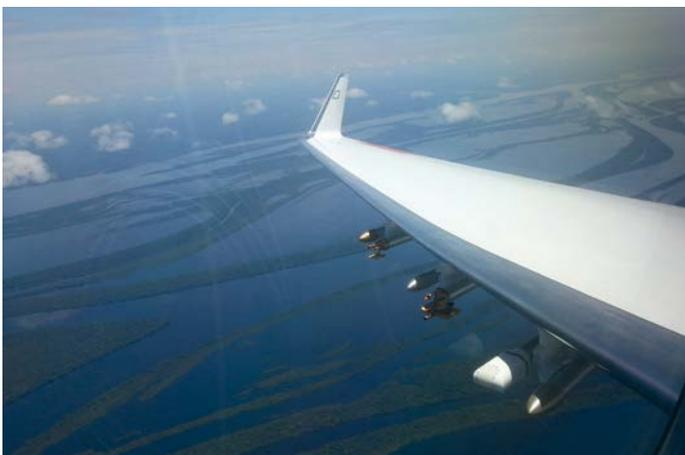
DLR's HALO research aircraft above the rainforest. Also on board: HAI, PTB's highly accurate humidity measuring instrument specifically developed for use in airplanes and in clouds.
