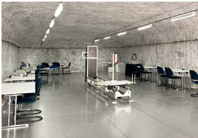
Low-dose calibration facility in PTB's underground laboratory UDO II
