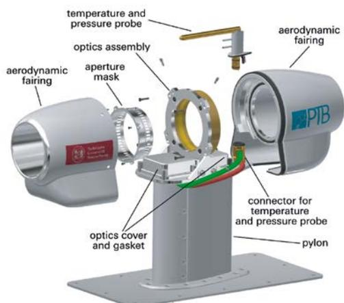
Laser hygrometer transfer standard for flux measurements on the new research aircraft of TU Braunschweig. (Figure: Felix Witt, TU Braunschweig)
