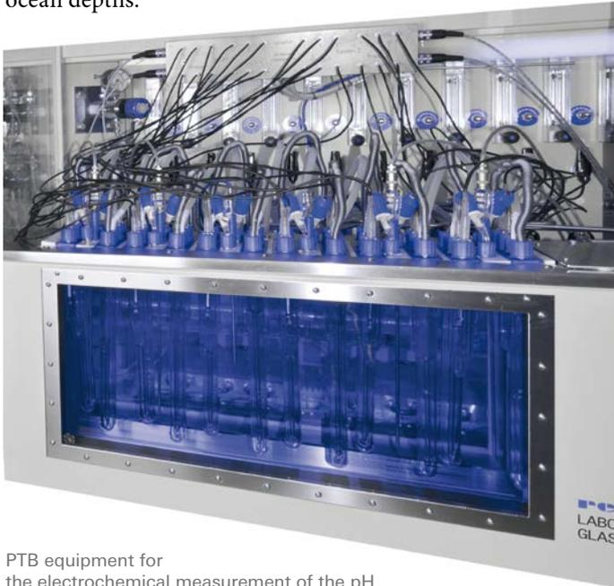
PTB equipment for the electrochemical measurement of the pH
