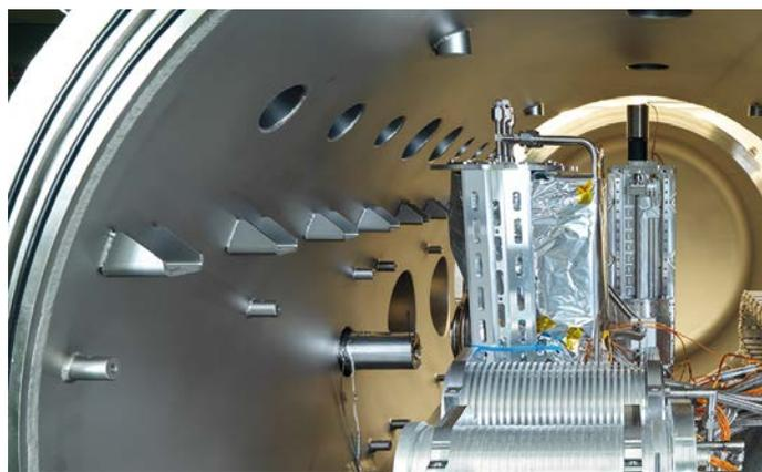
The interior view of the source chamber of the Reduced Background Calibration Facility 2. In the foreground: the reference blackbody radiators against which, for example, the FORUM and GLORIA reference sources are calibrated.
