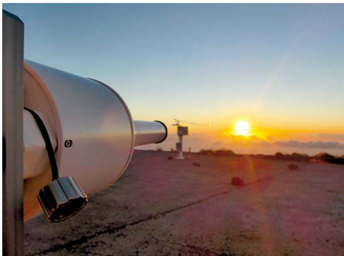
An array spectroradiometer characterized at PTB faces the rising sun at the Izaña Atmospheric Observatory (IZO) in Tenerife during an international comparison measurement campaign to determine the ozone column.
