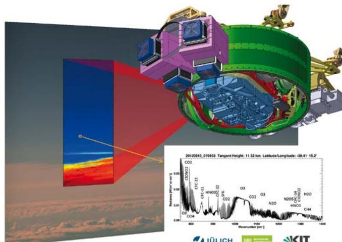
The GLORIA infrared Fourier spectrometer is regularly taken on the various missions of the German Aerospace Center's HALO research aircraft. It can carry out more than 16,000 spatially and spectrally resolved atmospheric observations simultaneously and is regularly recalibrated by PTB.
