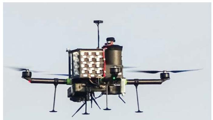
The ALICE quadcopter takes air samples that can then be further analyzed in the laboratory. In addition, it measures temperature and humidity profiles up to 1000 m altitude. (Photo: Astrid Lampert, TU Braunschweig)
