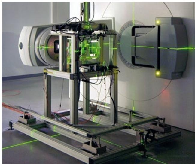
Measurement setup for the calibration of dosimeters in units of absorbed dose to water at one of PTB’s clinical linear accelerators.
