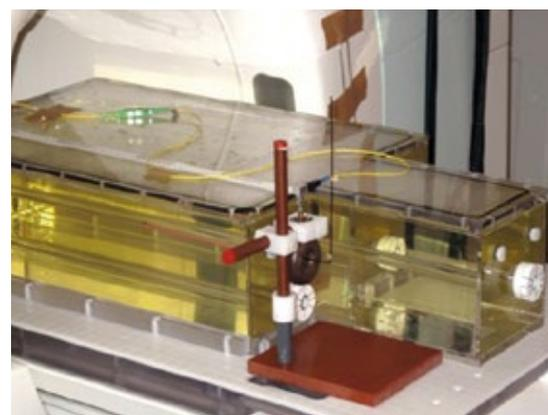
Phantom with a wire in the „shoulder“, together with a current sensor within the 3-tesla MR scanner of PTB
