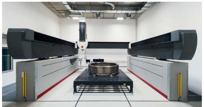
The large coordinate measuring machine enables the metrological traceability of large components (5 m × 4 m × 2 m measuring volume) for the first time.
