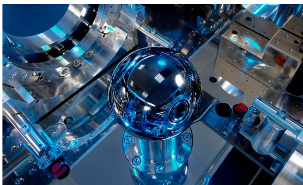
This silicon sphere weighs exactly one kilogram – down to the atom
