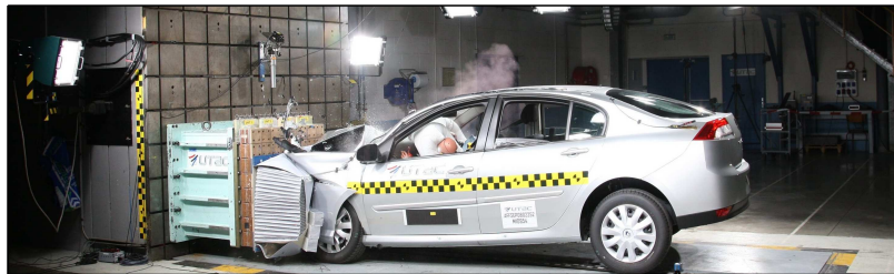
Figure 1: Example of a dynamic measurement involving the measurement of dynamic acceleration and shock force (photo Christophe Bertolin)
