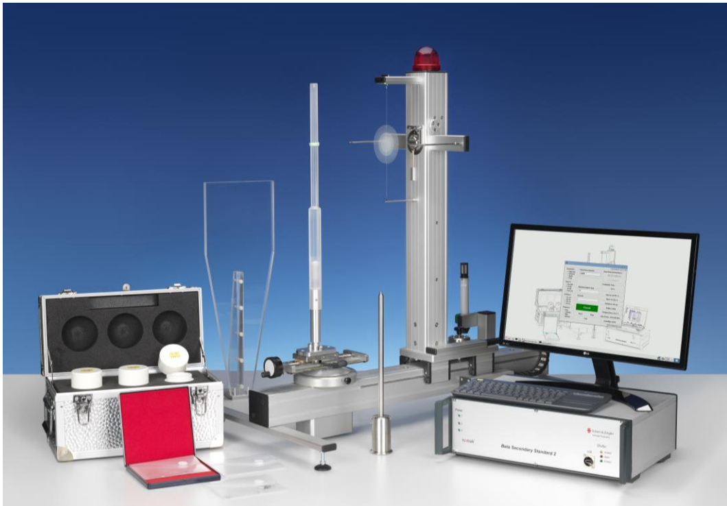
Figure 2. Photograph of the current BSS 2 model including the new ISO rod and ISO-equivalent slab phantom and an embedded mini-PC inside the control electronics.
