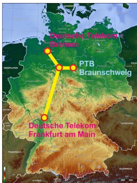
Figure 9. Scheme of the fiber optic time transfer network (proof of concept phase 3) between Deutsche Telekom and PTB.
