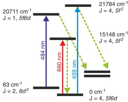
FIG. 1. Partial level scheme of  $\text{Th}^{2+}$ , showing the transitions relevant to our investigations. The levels are labeled by their energy in  $\text{cm}^{-1}$ , electronic angular momentum  $J$ , and the dominant configuration of the valence electrons. Laser excitation is shown with solid arrows. The detection is provided via fluorescence decay, indicated by dashed lines.
