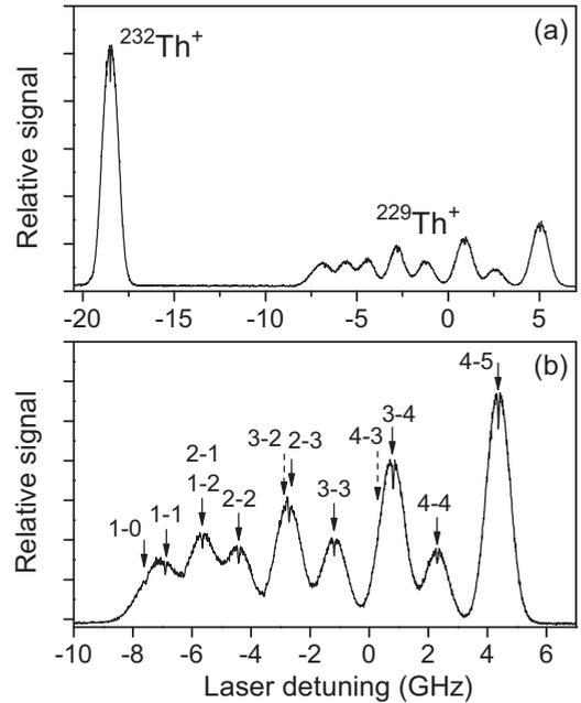
FIG. 1. (a) Fluorescence signal of the 402.0-nm line of  $^{229}\text{Th}^+$  and  $^{232}\text{Th}^+$  isotopes. (b) HFS signal of the 402.0-nm  $^{229}\text{Th}^+$  line. The detuning counts from the recalculated HFS centroid position of the  $^{229}\text{Th}^+$  isotope line. The components are labeled with the total angular momenta of lower and upper hyperfine levels. The dashed arrows in (b) show the recalculated positions of the  $3 \rightarrow 2$  and  $4 \rightarrow 3$  resonances.
