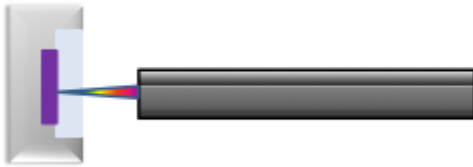
Figure 7: Scheme of the measurement principle of the confocal probe head on a WPVS cell. The wavelength of the light which is focused to the surface and reflected depends on the distance to the probe head. Its position is calculated from the spectral measurement of the surface reflectance.
