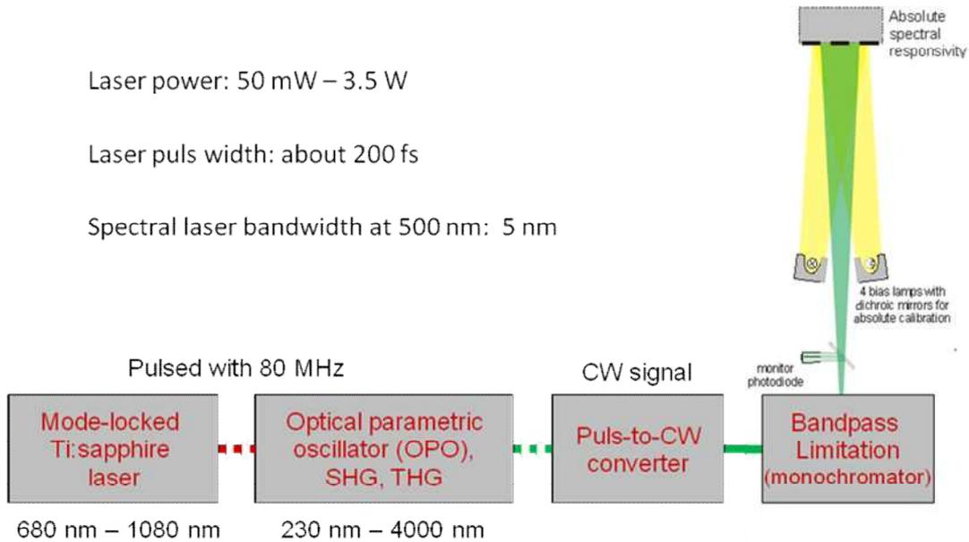
**Fig. 1:** Schematic diagram of the new Laser-DSR facility: The beam starts at a hands-free widely tunable mode-locked Ti:sapphire laser. Depending on the needed wavelength the beam passes through an optical parametric oscillator (OPO) and/or a second harmonic generator (SHG) or a third harmonic generator (THG). The pulsed signal is smoothed to a cw signal at a special pulsed-to-cw-converter developed at PTB. The bandpass is limited by a monochromator (see Fig. 2).
