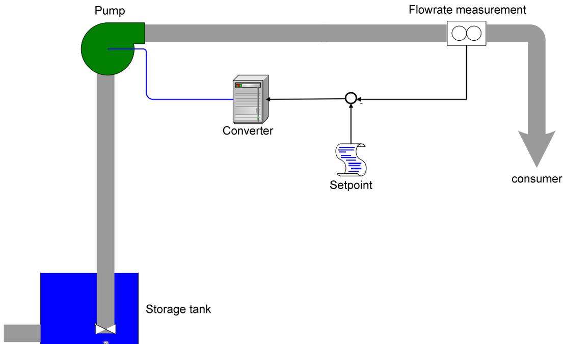
Figure 3: Adjustment of the flow rate by means of a frequency converter
