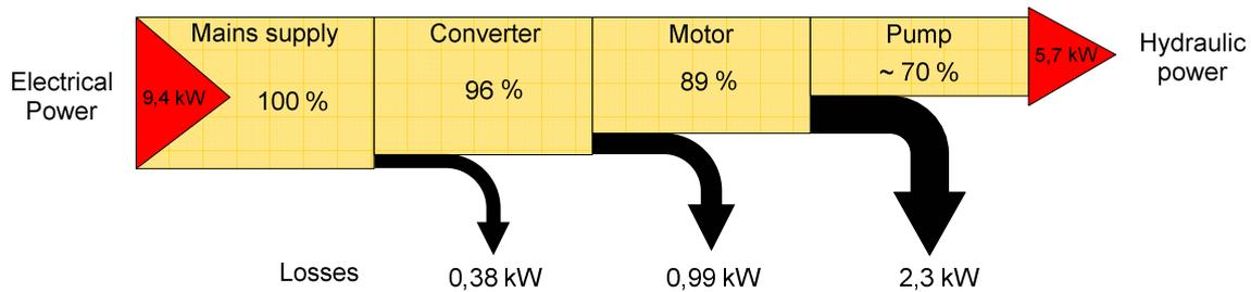
Figure 4: Loss sources during output adjustment of a pump by means of a frequency converter. Adjusted flow rate 30 m<sup>3</sup>/h, rated flow rate: 50 m<sup>3</sup>/h
