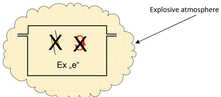
Figure 9: The principle of the type of protection "e"
