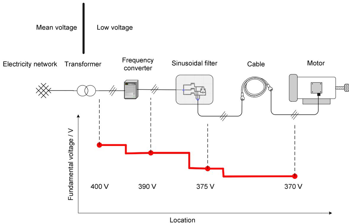
Figure 13: Voltage drops between electricity network and machine
