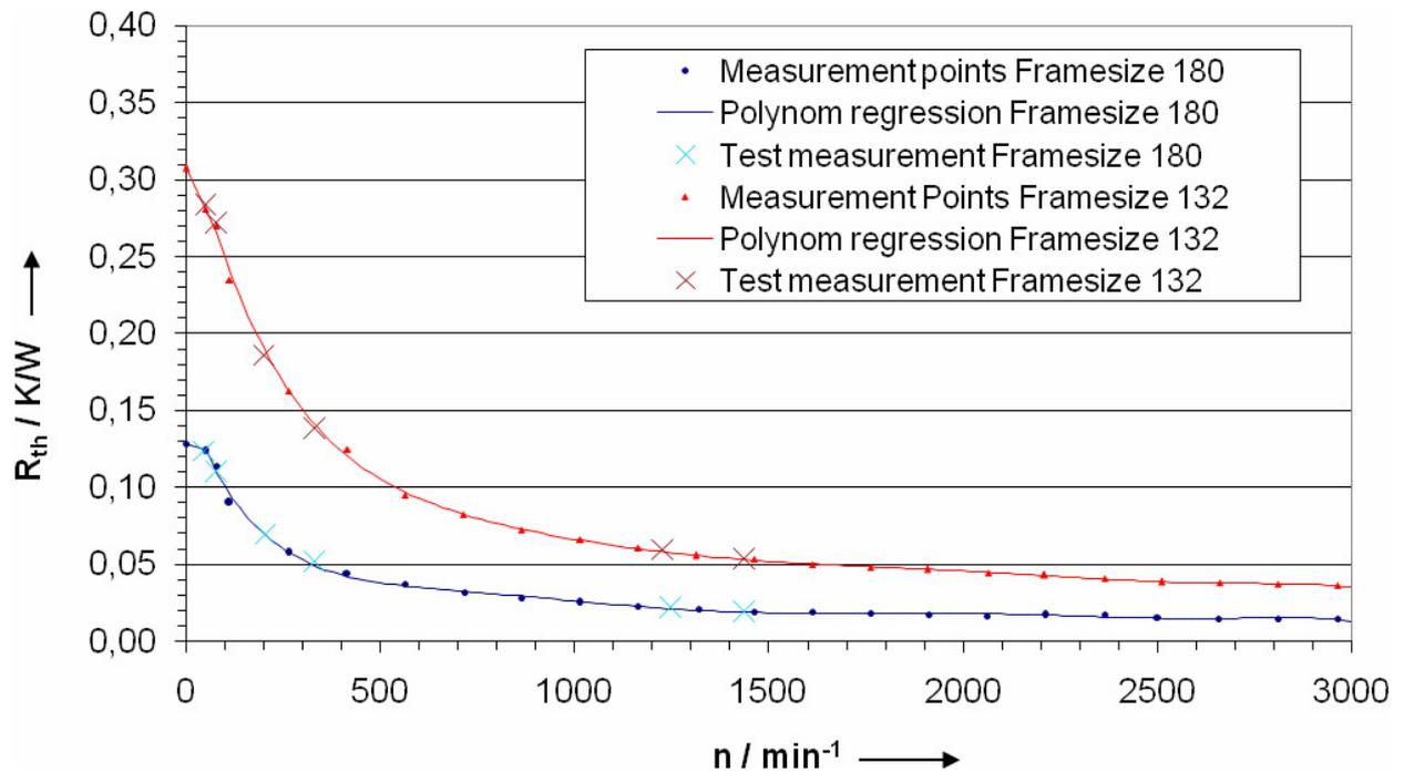
Figure 11: Development of the thermal resistance to the environment as a function of the speed
