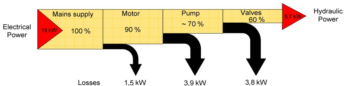
Figure 2: Sources of the losses in the flow rate adjustment at 30 m<sup>3</sup>/h by means of a flow reduction valve, design flow rate: 50 m<sup>3</sup>/h
