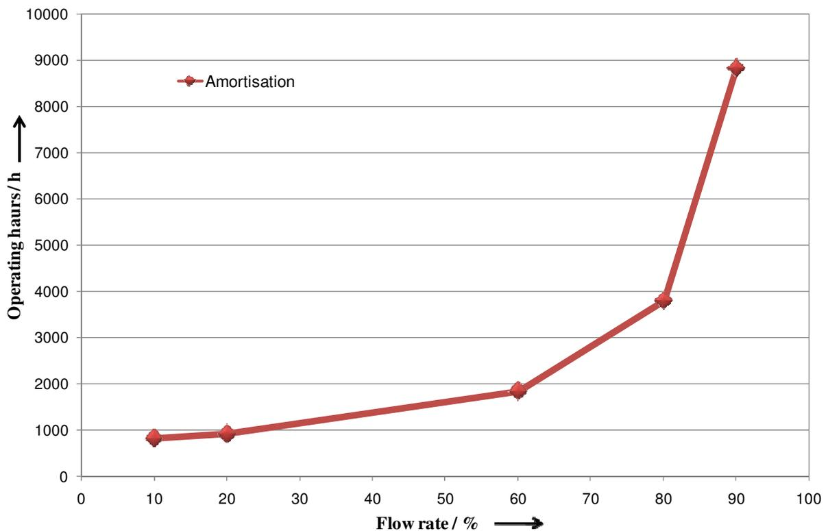
Figure 7: Amortisation time of the frequency converter as a function of the flow rate in percent related to the design flow rate of the pump
