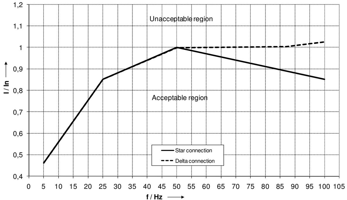
Figure 12: Speed-variable current limitation, from the EC type-examination certificate
