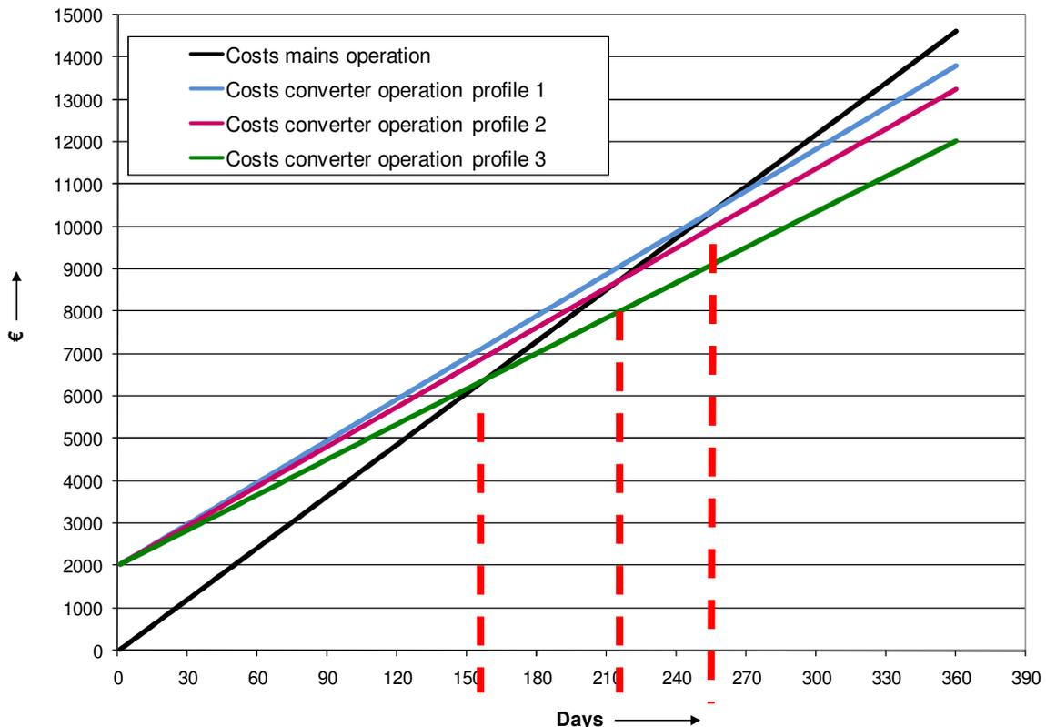
Figure 6: Development of the energy costs in the course of time for mains operation and for frequency converter operation.
