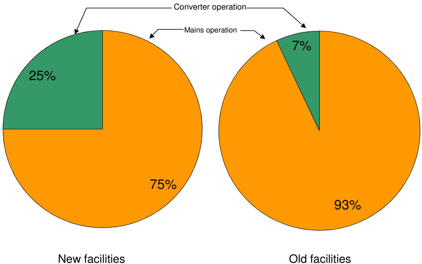
Figure 8: Share of converter-fed drives/motors in the chemical industry
