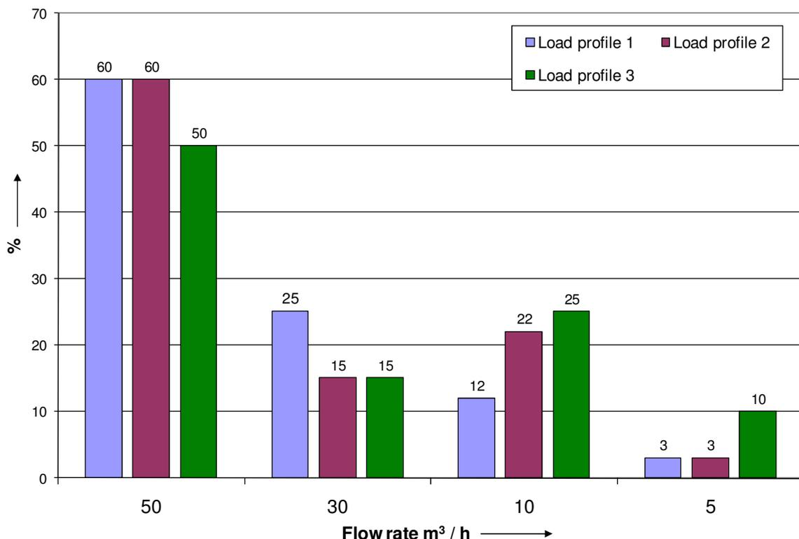
Figure 5: Assumed load profiles for the calculation of the amortisation times.
