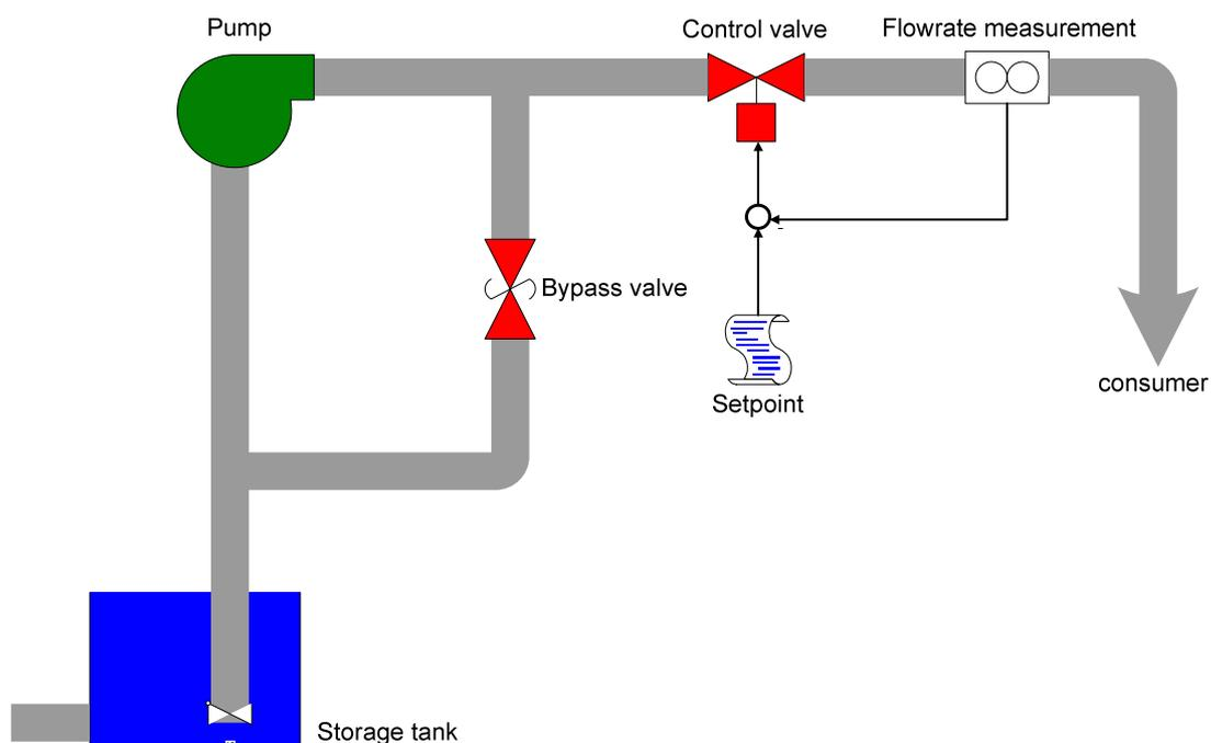
Figure 1: Adjustment of the flow rate by means of a flow reduction valve
