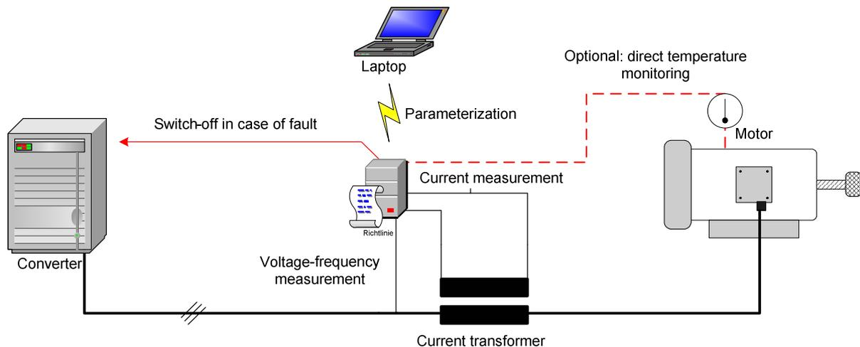
Figure 14: Supervision of the motor during converter operation
