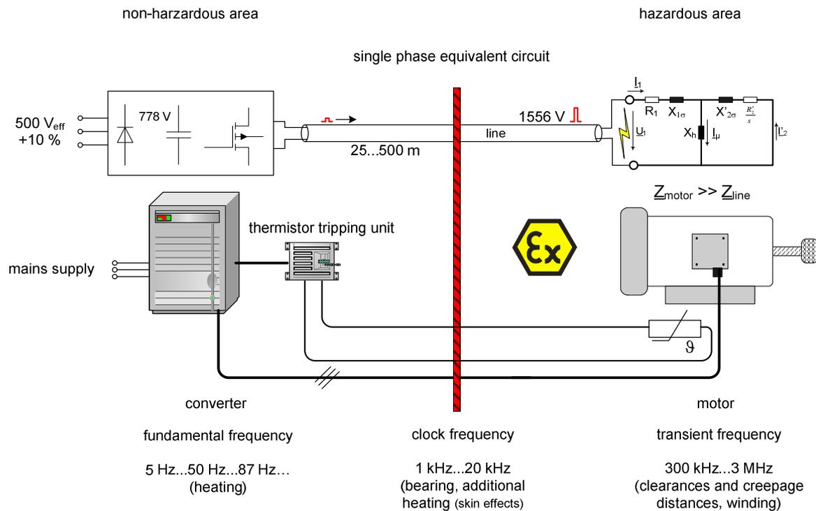
Figure 10: Development of transients on a frequency-converter-fed motor
