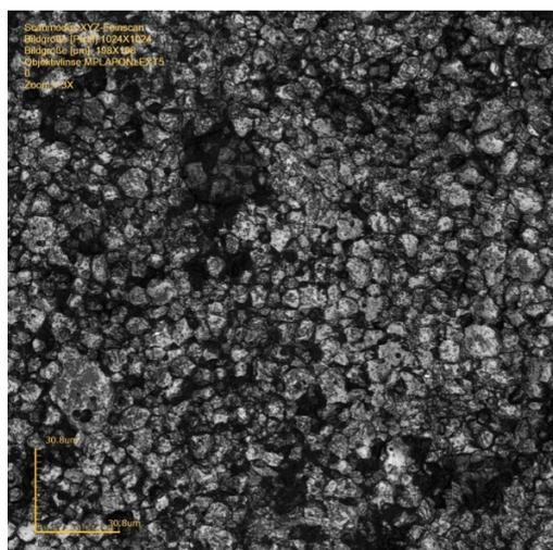
Fig. 5 CLSM of S2 magnet before corrosion (30 by 30  $\mu$ m)
