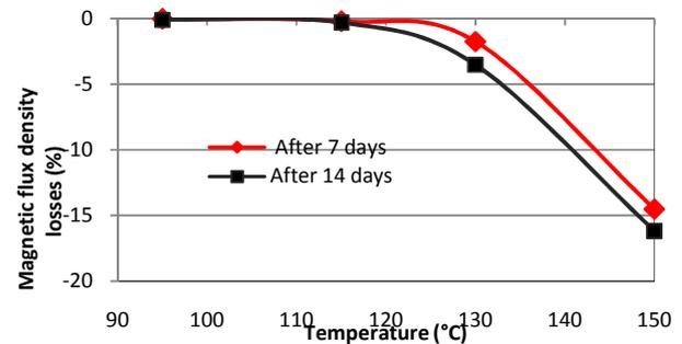
Fig. 7 Irreversible magnetic losses as a function of temperature for 7 and 14 days
