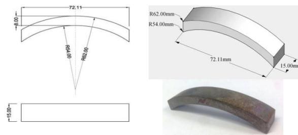
Fig. 1 Curved magnet with dimensions
