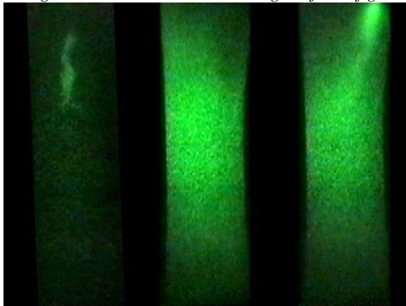
Fig. 6: Three discharges inside a vertical tube during the flow of gasoline
