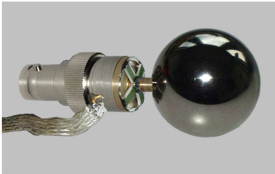
Fig. 3: Example of a high-frequency shunt resistance of 0.25 Ohm coupled to an oscilloscope
