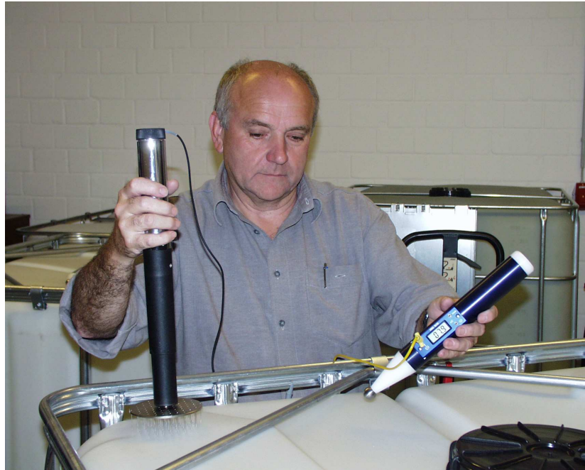
Fig. 2: Measuring the transferred charge with a coulombmeter in dry climate after charging with electrons spraying from needles on a potential of -70 kV (fakir electrode).
