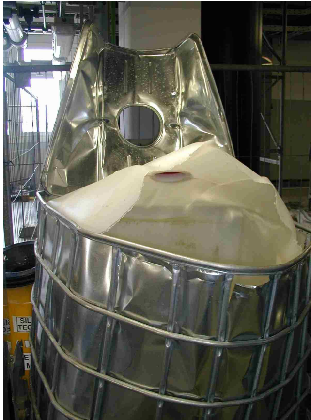
Fig. 1: 1 m 3 Container for flammable liquids after an explosion caused by static electricity
