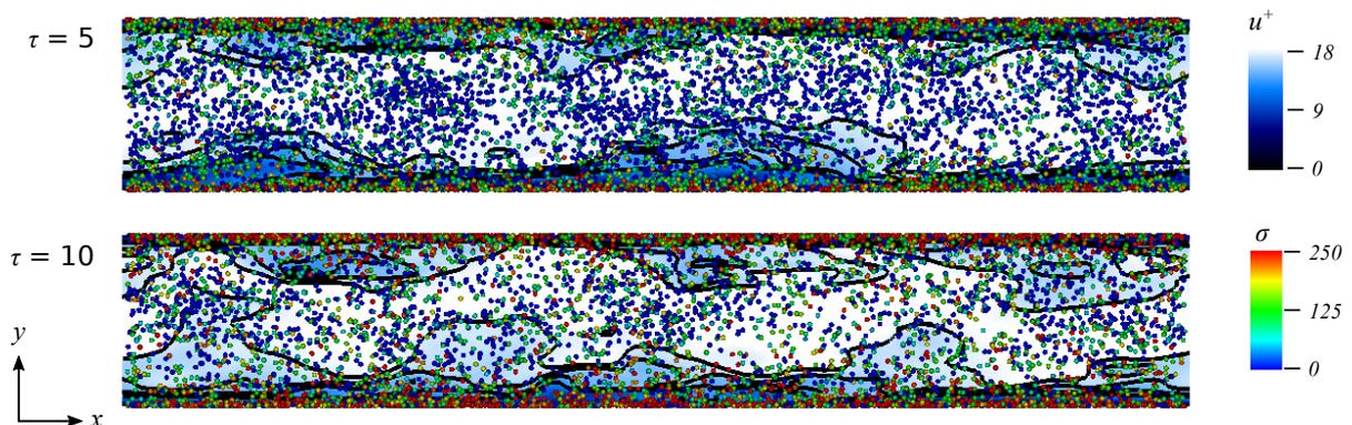
Figure 1: Instantaneous visualizations of the charging of particles in a channel flow. The black contours represent the isolines of the magnitude of the fluid velocity [1].
