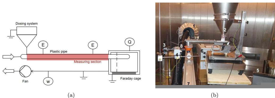
Figure 1: (a) Schematics and (b) photo of the experimental facility at PTB [1]. (1) Faraday cage, (2) dosing system, (3) Voltmeter and amplifier, (4) flow meter, (5) frequency converter, (6) control unit of the dosing system, (7) support structure, (8) two electric field strength meters.
