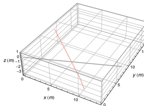
**Fig. 1** Two tubes (gray and red line) running below the SENSYS-test area
