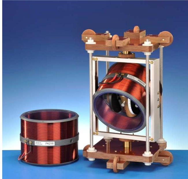
**Fig. 2** Picture of two identical rotatable coils PK215 (here on the right hand side mounted within a trolley stand for the positioning of the coil in the tubes running below the SENSYS-test area) and PK216 (on the left hand side without frame) for the simulation of the stray magnetic fields of UXBs.
