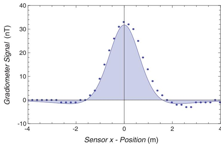
**Fig. 3** Profile of the gradient signal (full line) calculated by use of Equ. (1) for a magnetic moment of  $1.185\text{Am}^2$  in a depth of the magnetic moment below ground level of 1.39m. The discrete experimental data points plotted above were selected from an exploration on the test ground with fluxgate gradient sensors by use of the coil PK215 shown in Fig. 2.
