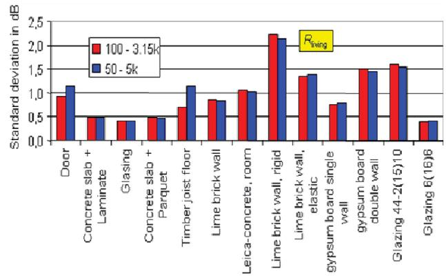
**Figure 5:** Standard deviation of  $R_{living}$  of different Round-Robin tests. Blue: full frequency range from 50 to 5000 Hz regarded. Red: only 100 to 3150 Hz regarded.
