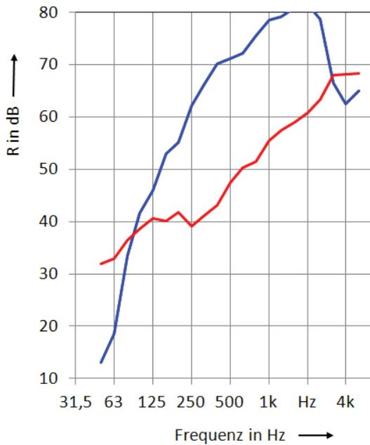
**Figure 3:** Examined sound reduction index spectra. Blue: lightweight double wall. Red: masonry wall
