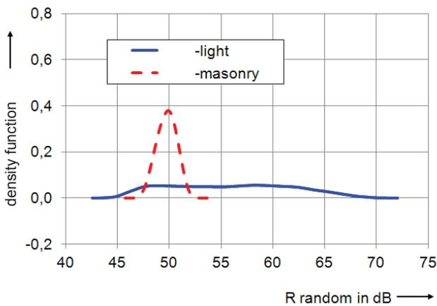
**Figure 4:** Resulting sound reduction index distributions for the walls in Figure 3.
