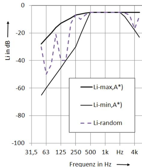
**Figure 2:** Limiting curves for the applied source spectra to calculate the A-weighted sound power level differences of building elements to represent their sound reduction performance. Based on [4].
