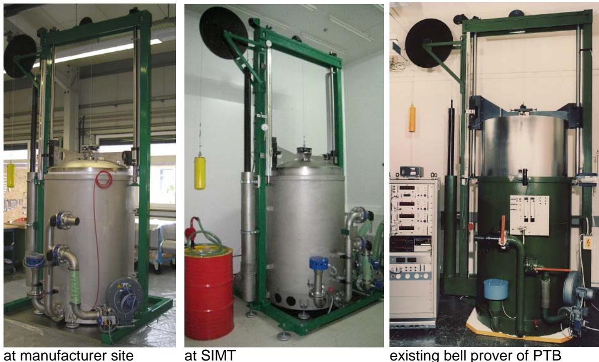
Fig. 1: Photos of the new constructed the bell prover left at manufacturer site middle at Shanghai Institute of Metrology and Testing Technology (SIMT) as well as the PTB bell prover (right)
