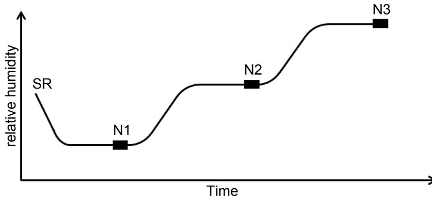
**Figure 7:** Visualisation calibration sequence B2: Relative humidity value of the calibration device (reference value) as a function of time
