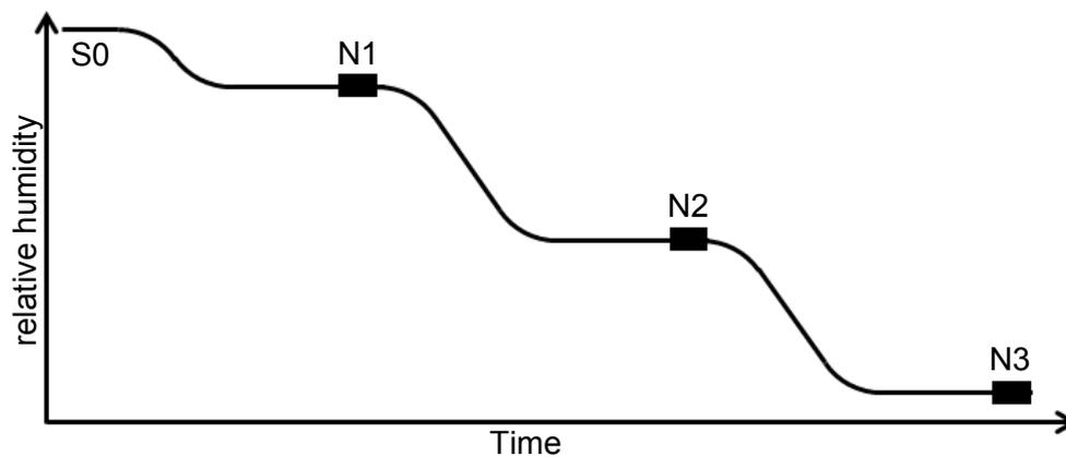
**Figure 8:** Visualisation calibration sequence C1: Relative humidity value of the calibration device (reference value) as a function of time
