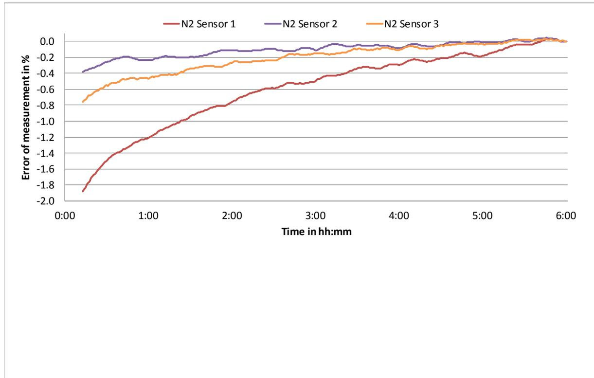
**Figure 17:** Measurement deviations of the relative humidity of 3 humidity sensors as a function of time at calibration point N2
