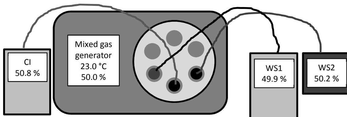
**Figure 12:** Schematic representation calibration set-up
