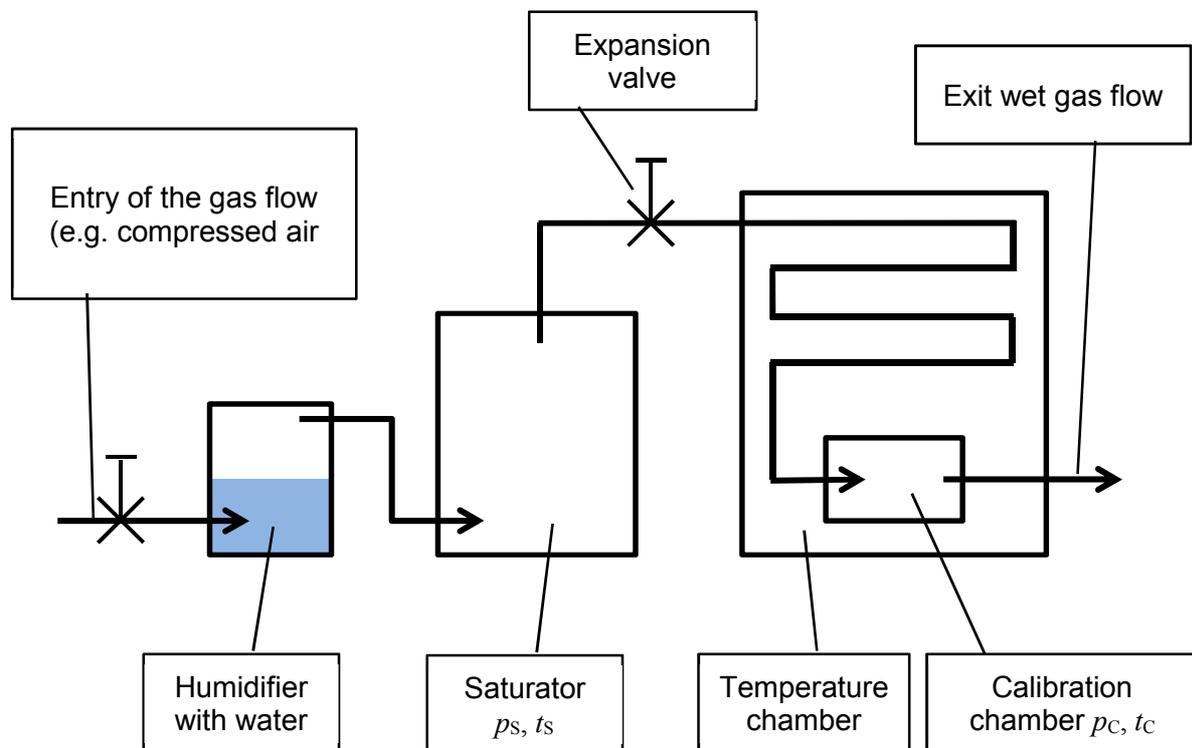
**Figure 2:** Schematic representation of a two-pressure/two-temperature humidity generator with saturation above water
