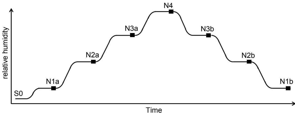
**Figure 4:** Visualisation calibration sequence A1: Relative humidity value of the calibration device (reference value) as a function of time
