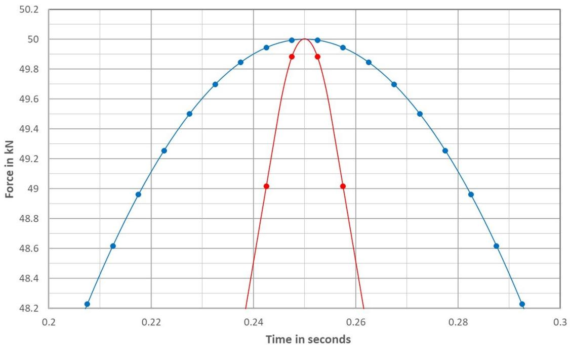
**Figure 4:** Sampling of a sinusoidal and triangular oscillation with 200 sampling points per cycle
