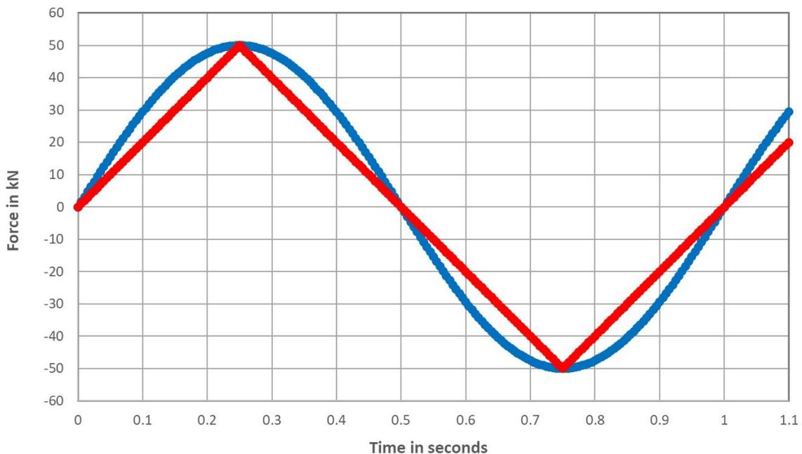
**Figure 2:** Signal curve for sinusoidal and triangular loads
