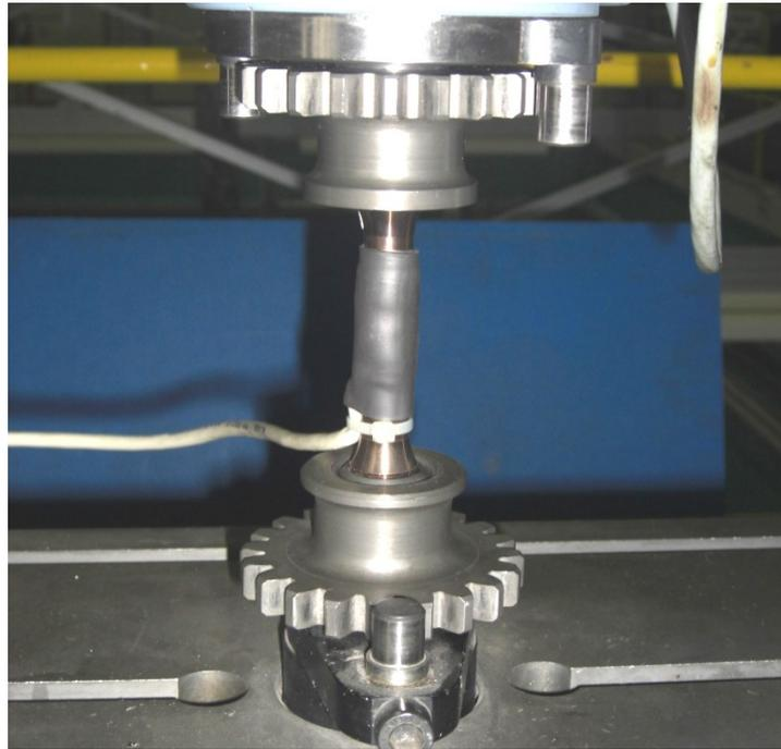
**Figure 1:** Built-in applied round specimen including clamping tool
