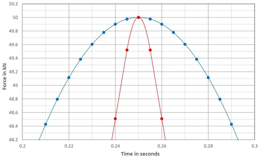
**Figure 3:** Sampling of a sinusoidal and a triangular oscillation, 200 sampling points per cycle, signal peaks rounded, data point on vertex
