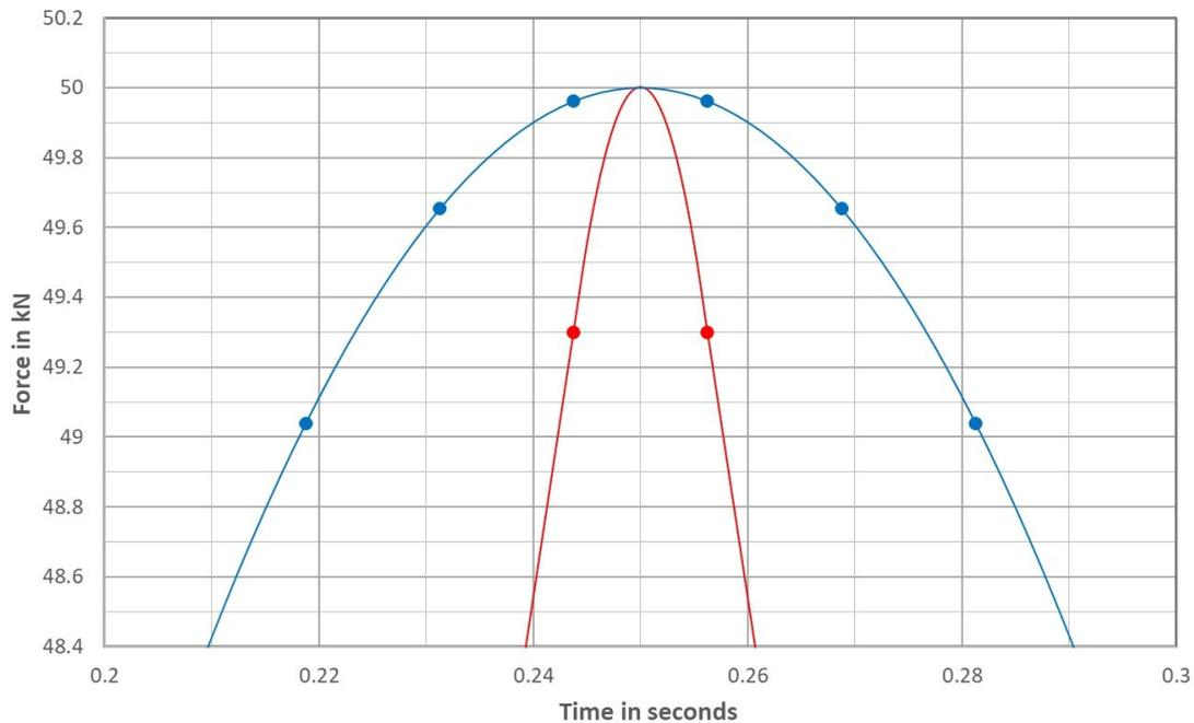
**Figure 5:** Sampling of a sinusoidal and triangular oscillation with 80 sampling points per cycle
