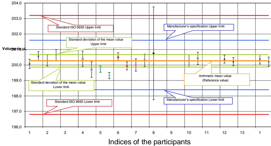
Figure 4: Graphical representation of the measurement results for a multi-channel piston-operated pipette with a variable volume (Transferpette S 20  $\mu\text{L}$  - 200  $\mu\text{L}$ ; channel 1; tested volume 200  $\mu\text{L}$ )
