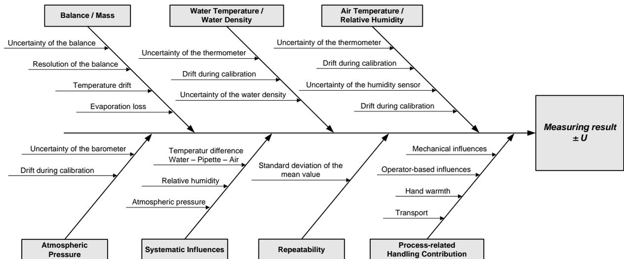
Figure 5: Cause-effect-diagram for the calibration of different piston-operated pipettes with air cushion
