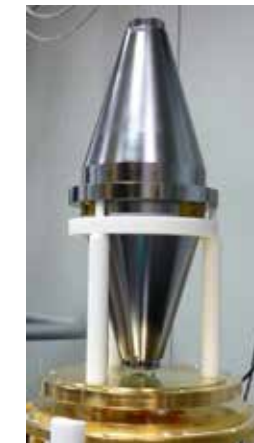
Fig. 1: Vibration insensitive mounting of the 21 cm long single-crystal silicon cavity.
