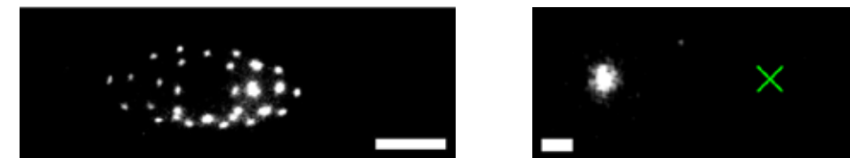
Fig. 1: Left: A single \text{Ar}^{13+} ion sympathetically cooled by several \text{Be}^+ ions. White scale bar denotes 100 \mu\text{m} . Right: A single \text{Ar}^{13+} ion (position marked by cross) sympathetically cooled by a single laser-cooled \text{Be}^+ ion. White scale bar denotes 20 \mu\text{m} .
