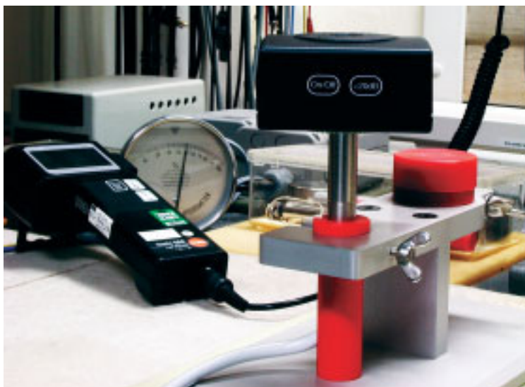
Figure 7: Sound calibrator (black box, foreground, right) attached to a reference microphone (silver, vertical cylinder, foreground, right)
