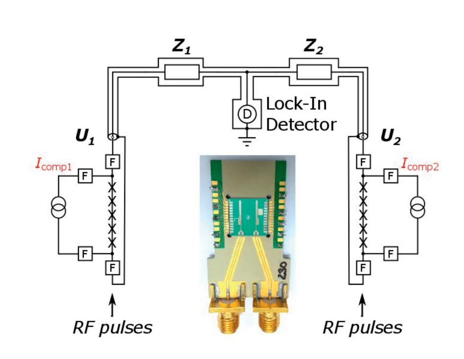
Two independent pulse-driven arrays arranged on one chip.
