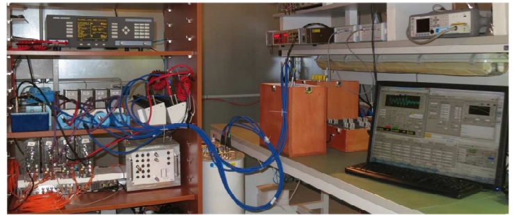
FD-DA bridge (left), reference standards (middle), DUT (right)
