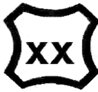
figure 2: mark of the year of verification (xx = the two last digits)
