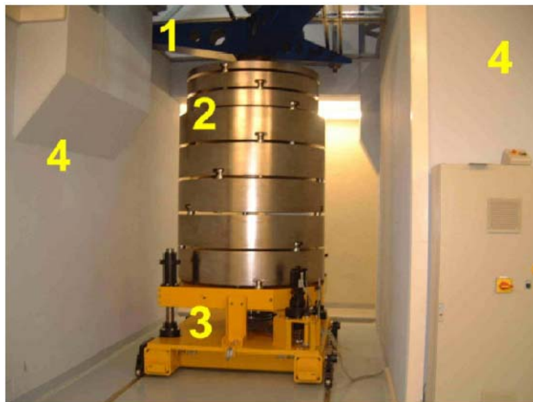
Figure 3. 30-tons balance: view of the calibration weights loading system
