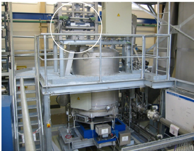
Figure 4 3-tons weighing system with fluid diverter (highlighted by the circular marker)
