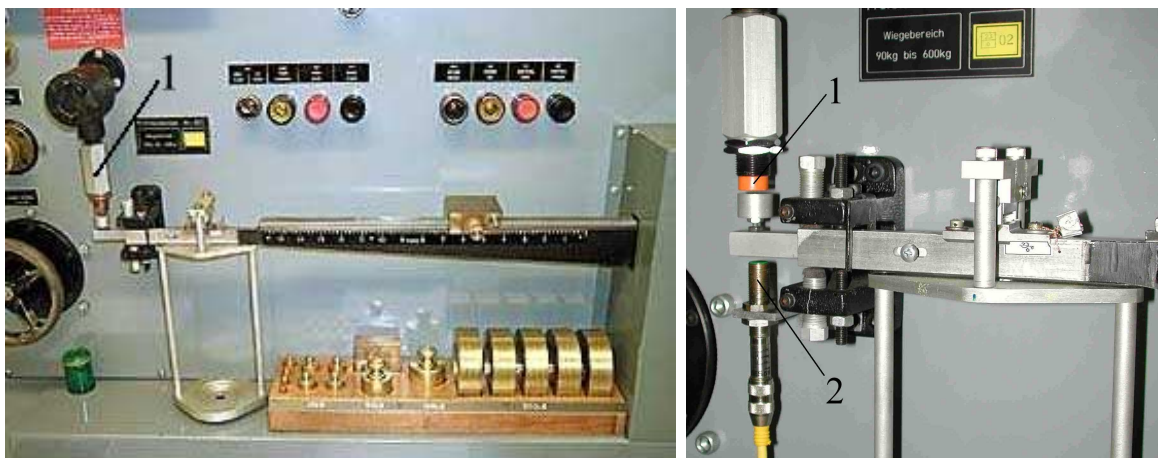
a) Figure 3. Compound beam weighing system a) Detail view of tare beam (with "standard" proximity switch 1 only) b) Tare beam with additional zero position proximity switch 2 (reproduced with permission of KEM Küppers Elektromechanik GmbH, Karlsfeld, Germany)
