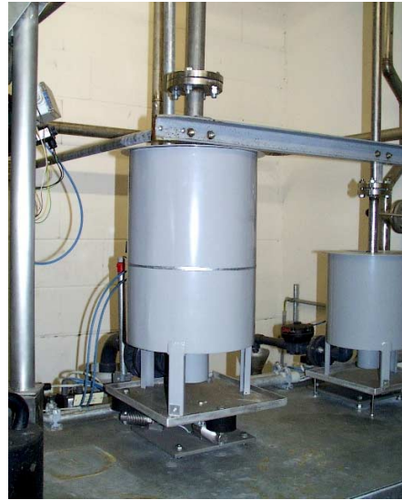
Figure 4. Gravimetric reference with immersed inlet pipe and flow deflecting plate a) Principle of function b) 40-kg balance of a dynamic weighing calibrator (Courtesy of Rota Yokogawa GmbH, Wehr, Germany)
