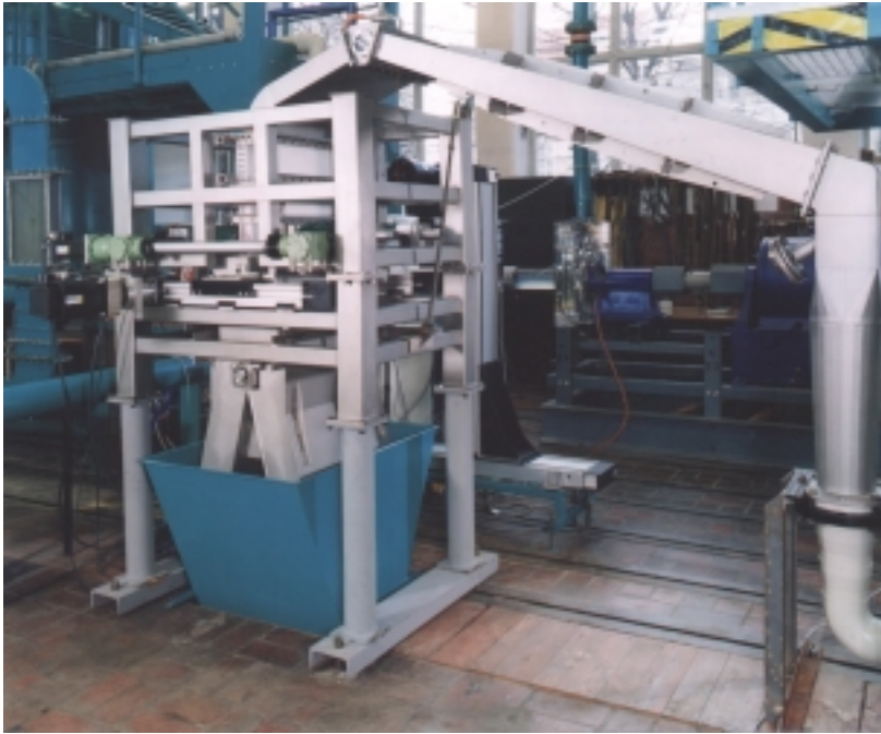
Figure 7. Test installation of the DN 150 mm diverter prototype
