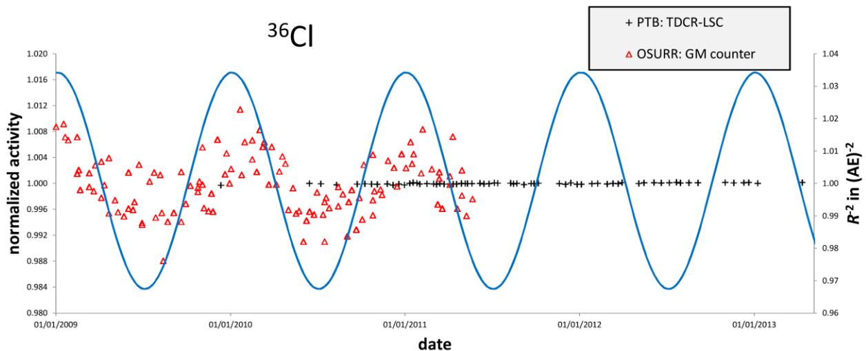
Fig. 1: The normalized activity as a function of time shows no dependence on the season in PTB's data, contrary to the data obtained at the Ohio State University Research Reactor (OSURR). The blue line represents the reciprocal square of the distance between the Sun and the Earth, expressed in the astronomic unit (AE).
